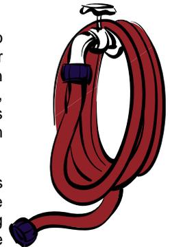
Backflow prevention is accomplished by installing a device that prohibits water from backflowing from one area to another. The backflow occurs when there is negative pressure in the line and water is sucked from one source to another. This means that water from an unprotected lawn sprinkler system may be sucked into the water lines in your home and contaminate your drinking water. Unknowingly drinking the contaminated water could result in sickness or even death.
